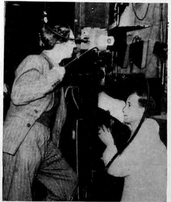
Engineers in Baird laboratory demonstrate "cine-televisor"; 30 seconds from scene to film to receiver
